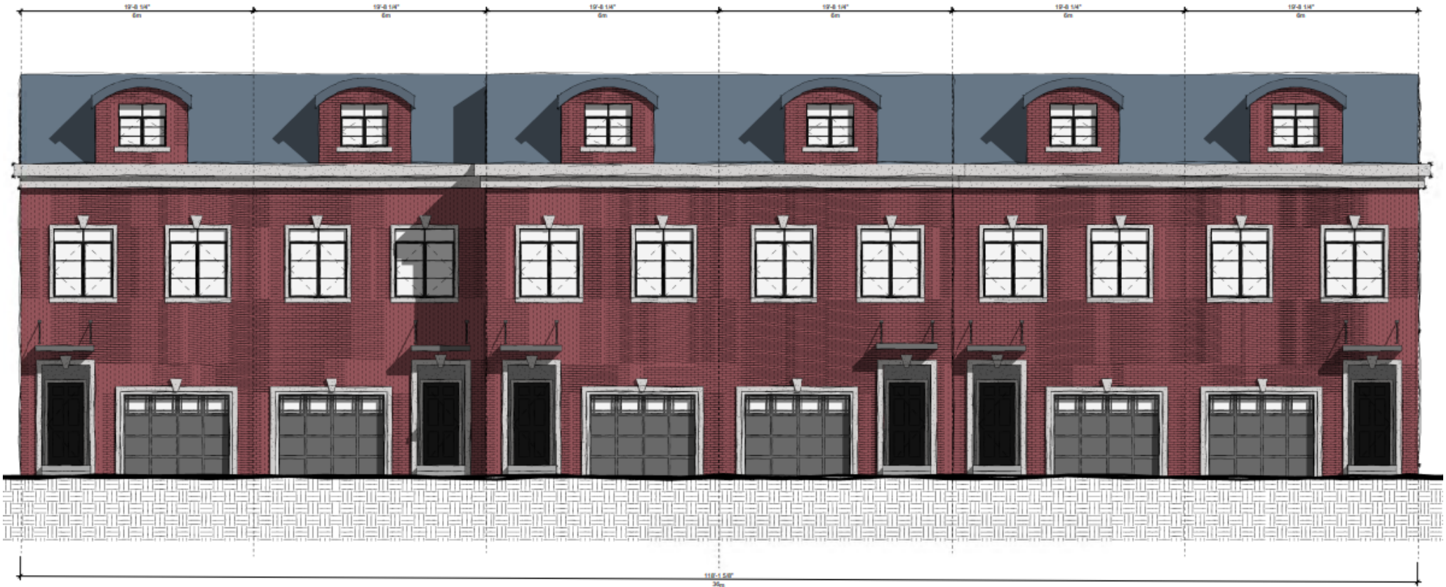
TYPICAL ELEVATION 6 UNIT ROW 1/4" = 1'-0"
